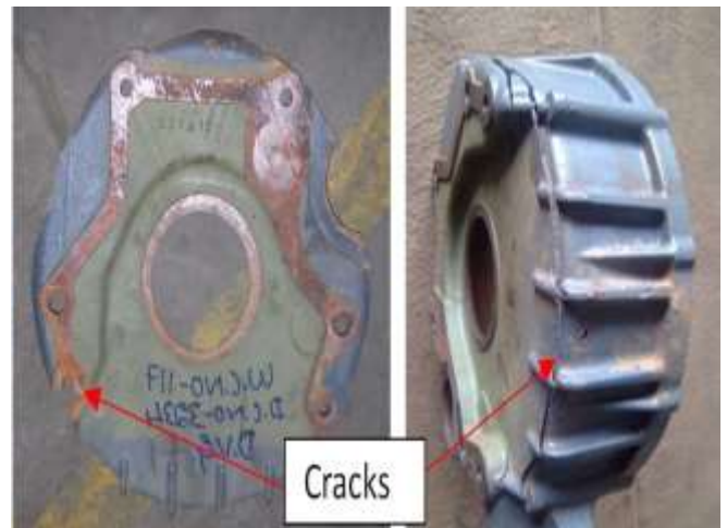
Fig. 1 - Crack in Flywheel housing
